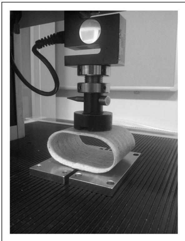
**Figure 3.** The material testing machine (Iloyd Ir30k, Iloyd instruments, southampton, uk).
